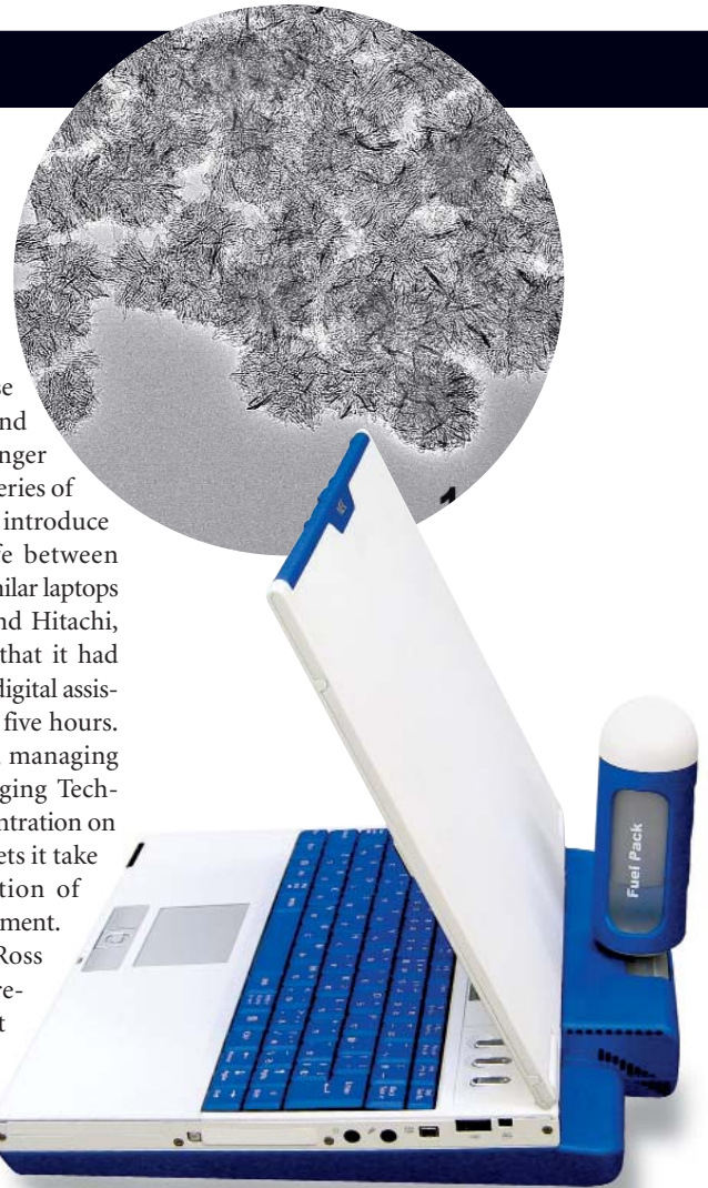
NEC used carbon nanohorns (inset) in fuel cell electrodes to provide longer life to a laptop powered by a methanol cartridge.
